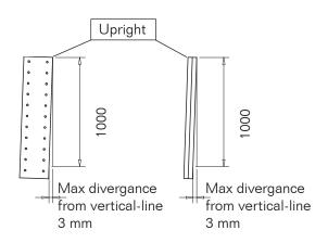
Max gradient of an unloaded upright 3 mm/m
