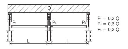
Q = Equal distributed load P = Load at each arm
