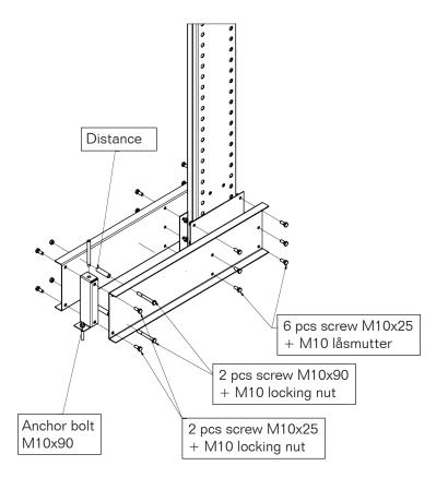
Tightening Torque Screw M10 8.8 Lock nut M10 class 8 Tighten screw joints for good contact Max tightening torque 47 Nm
